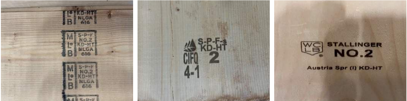
Delivered price is not the only variable quality is too. A series of different piles of lumber in a Maine Manufactured Housing Company: Maritime Lumber Bureau (MLB); CIFQ is the Quebec grading agency, and the third is obvious.
