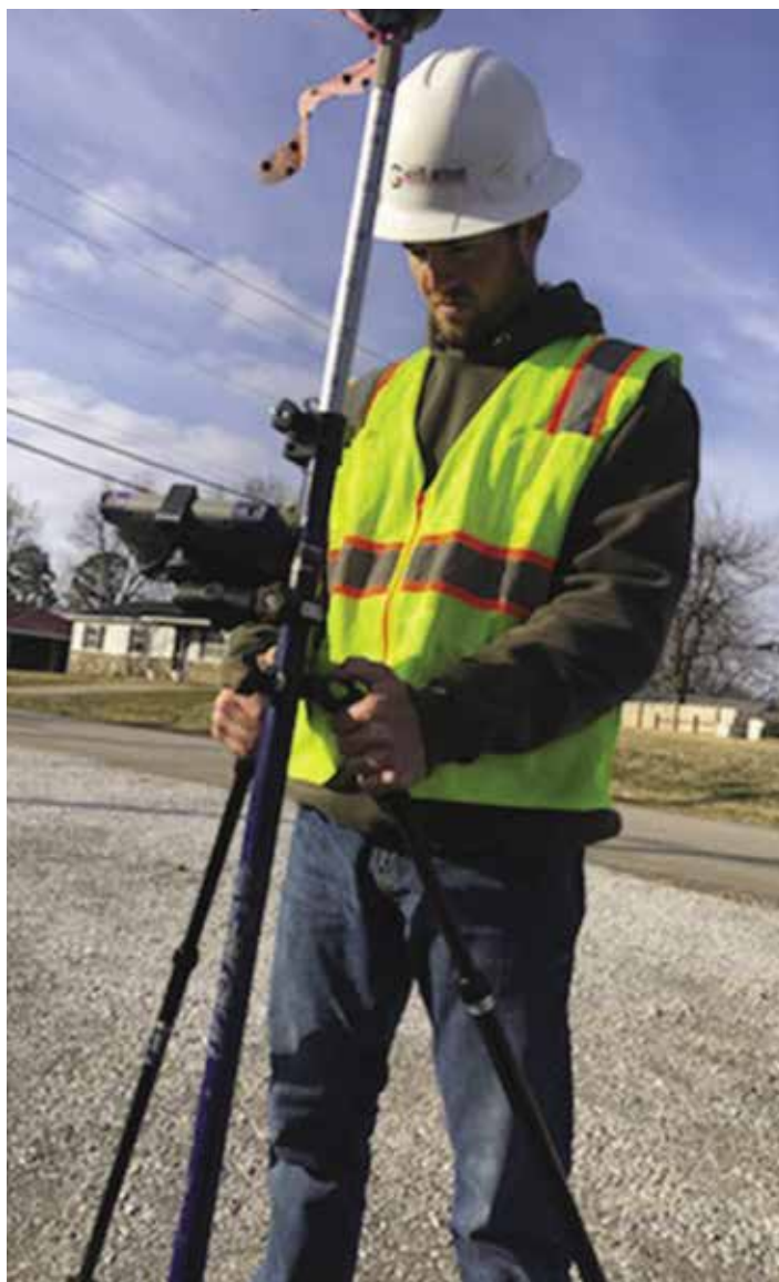
Evan Horne of the Civil Group, LLC in Florence calibrates his hyper accurate GPS in preparation for a survey.
