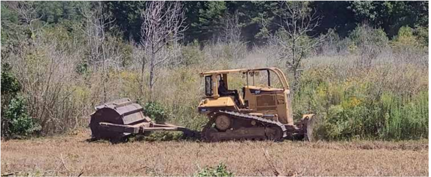
Cut-over sites quickly re-vegetate and can significantly slow the production of the tree planters. This landowner had to incorporate drum chopping into his site preparation efforts to allow access for planters before they would agree to plant.
